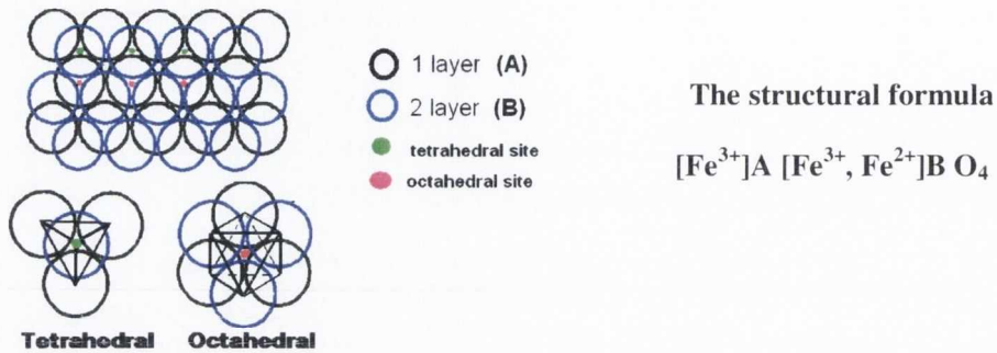
Figure 1.4. Structural formula of magnetite ( \text{Fe}_3\text{O}_4 ), where iron exists as \text{Fe}^{2+} , which preferentially occupies the octahedral site and \text{Fe}^{3+} , which shows no preference and occupies both the tetrahedral and octahedral sites.
