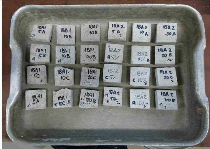
Figure 3-13: Representative samples used for testing specific heat for IBA 1 and IBA 2.
