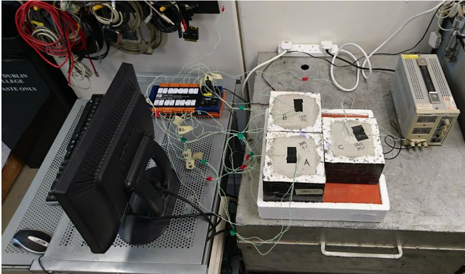
Figure 3-12: Thermal conductivity test set-up.
