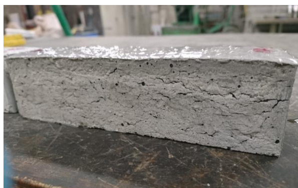
Figure 4-15: Specimen produced with IBA 2 – coarse after demoulding (at 72 hours).
