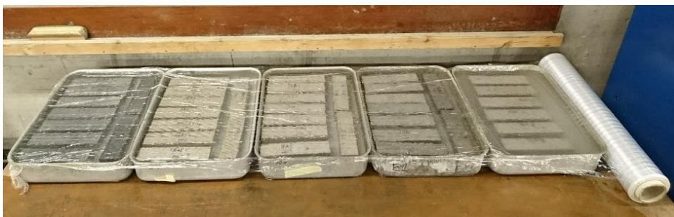
Figure 3-14: Samples immersed in saturated MgSO 4 solution.
