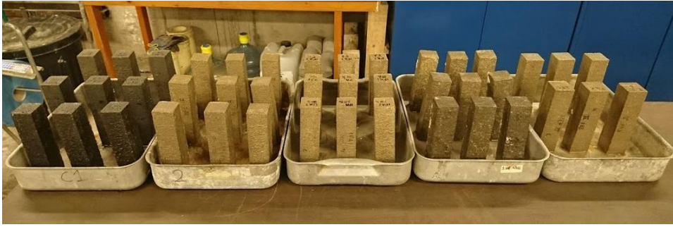
Figure 3-15: Specimens allowed to drain after immersion period.
