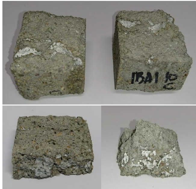
Figure 5-15: Salt precipitated within IBA 1 specimens. IBA 1 10% (top) and IBA 1 20% (bottom).
