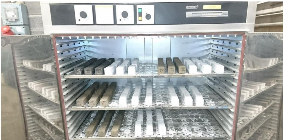
Figure 3-16: Samples maintained in oven for 24h after draining.
