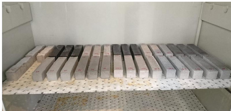
Figure 3-6: Prismatic test specimens for strength development tests.
