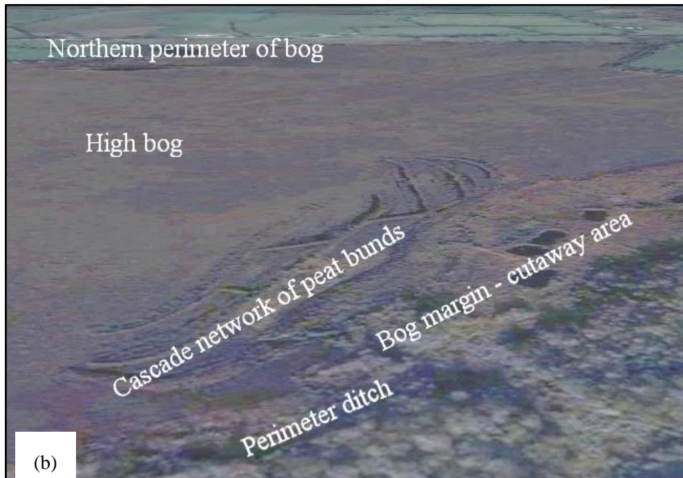
Fig. 4. Cascade network of peat bunds near south-eastern margin of Raheenmore raised bog, County Offaly, Ireland: (a) schematic diagram; (b) terrestrial image
