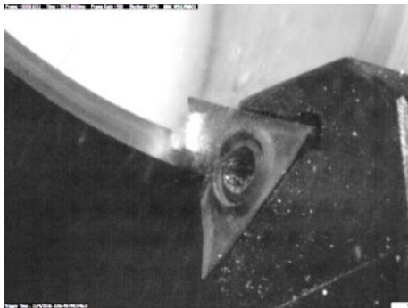
c) N 2 cold sprayed, no heat treatment. Very small chip formed
