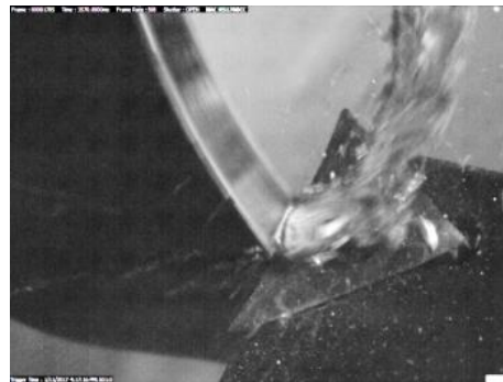
f) He cold sprayed, annealed. Thick discontinuous chip formed
