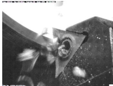
d) N 2 cold sprayed, annealed. Dust and small chip fragments formed
