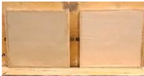
Fig. 4 Portland stone slabs rendered with 10 mm mortars in table 4.
