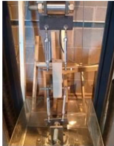
Fig. 5 Set up of pull-out test to measure bond strength between Portland stone and mortar.
