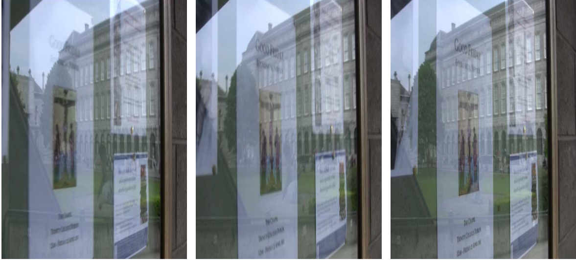
Figure 7.1: From left: Frames 1, 10, 20 from a sequence containing reflection of a building superimposed on paper posters. In this sequence the building is moving to the left while the posters are moving to the right. This generates two motions per pel.
