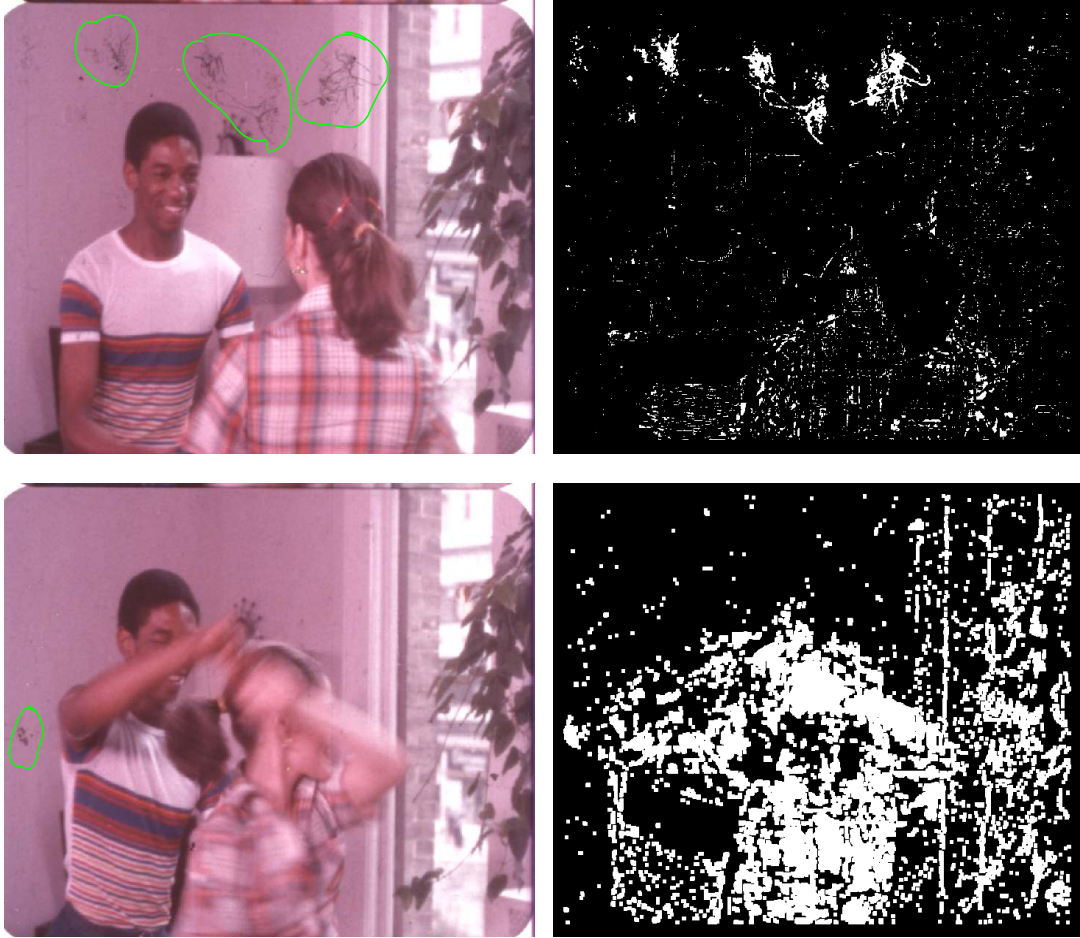
Figure 3.1: Left, from top: Frames 58 and 78 for a corrupted image sequences with blotches shown in green. Right: Corresponding SDIp detections. Here E_t is fixed to 5. For frame 78 the actors are moving quickly. This generates high false blotch detection rate.
