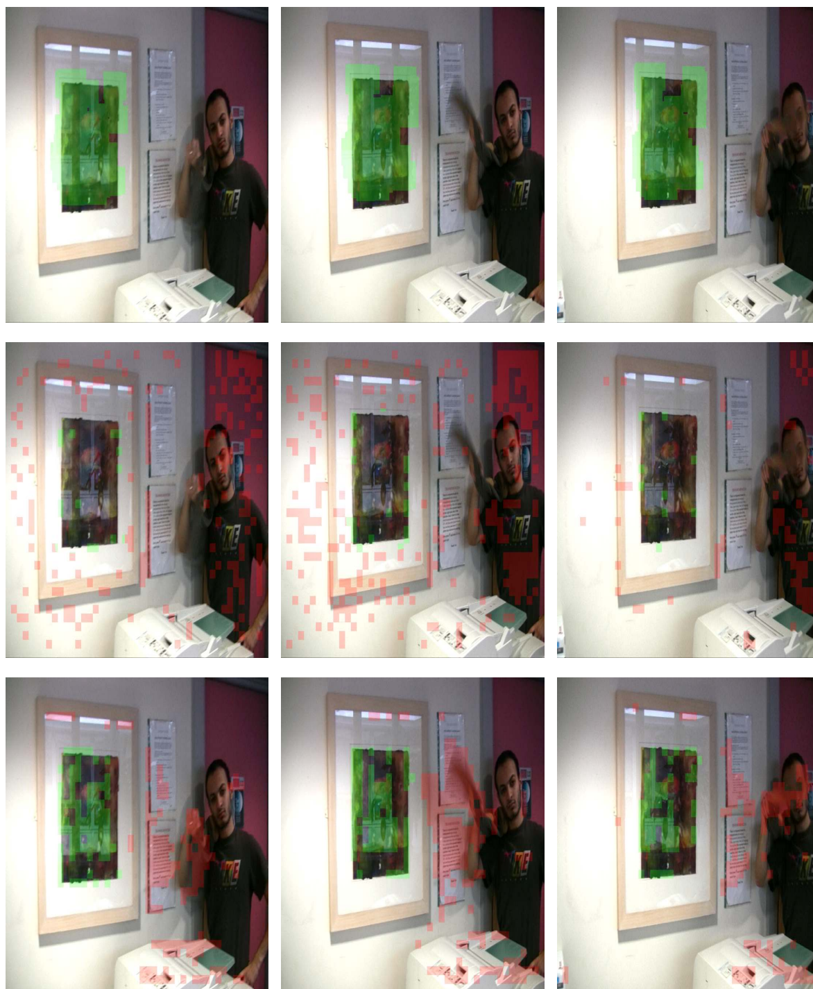
Figure 6.18: Reflection detection on SelimC using, from top; FEAPARD-F, SHARPNESS and DFD respectively. Correct detections are shown in green while false detections are shown in red. The pathological motion generated by the actor's hands is rejected by FEAPARD-F but detected by DFD.
