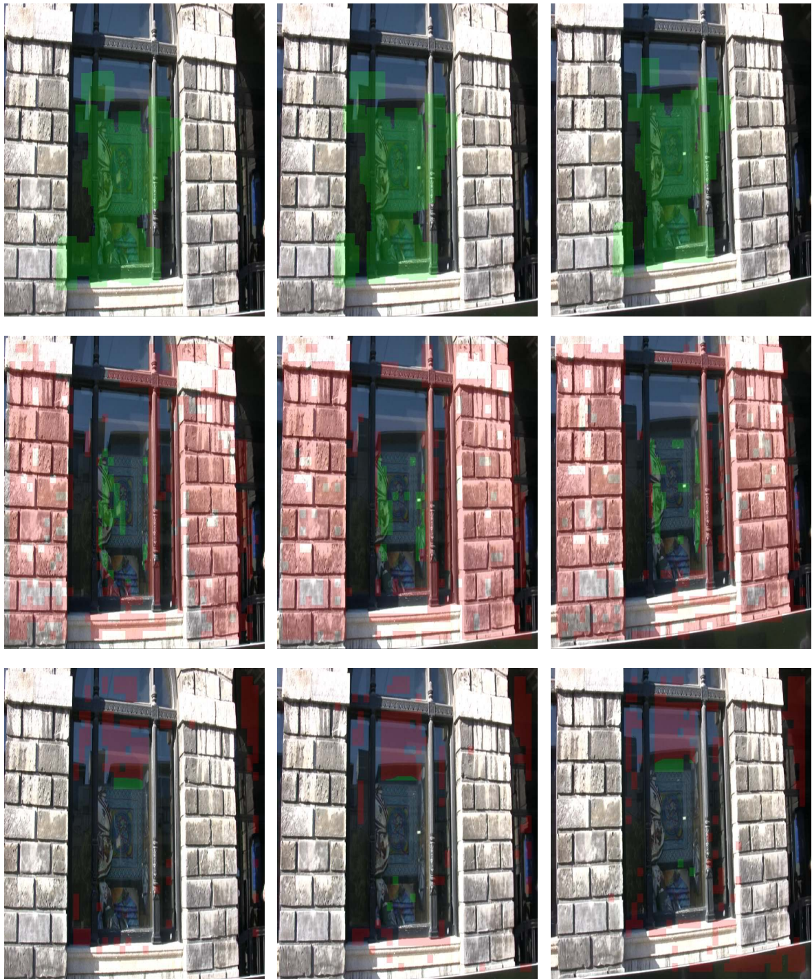
Figure 11.3: Reflection detection on BuildOnWind1 using, from top; FEAPARD-F, SHARPNESS and DFD respectively. Correct detections are shown in green while false detections are shown in red. SHARPNESS misclassifies flat areas as reflection.
