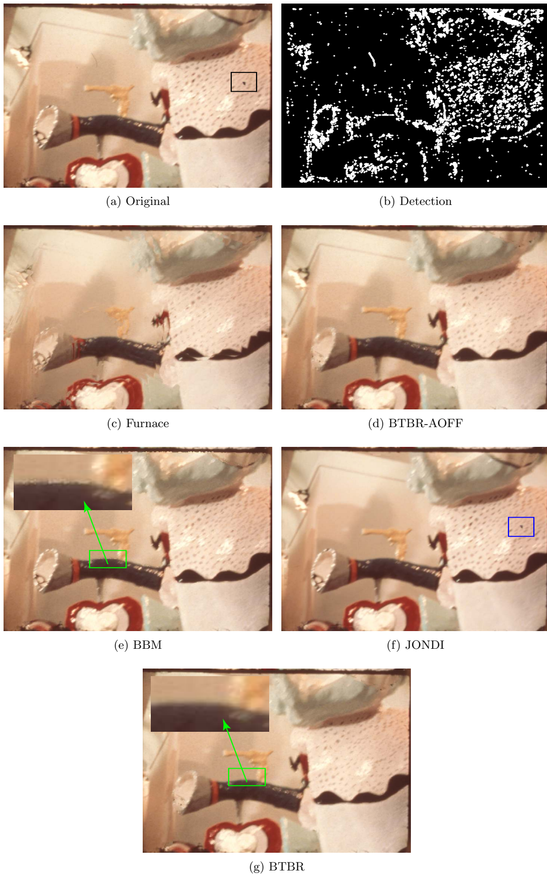
Figure 5.13: In clockwise direction: Frame 32 of ArtB1, its SDIp mask and reconstruction using different techniques. Blotches are shown in black boxes. JONDI failed in removing a very dark corruption (shown in blue) while BBM generates noisy results (shown in green).
