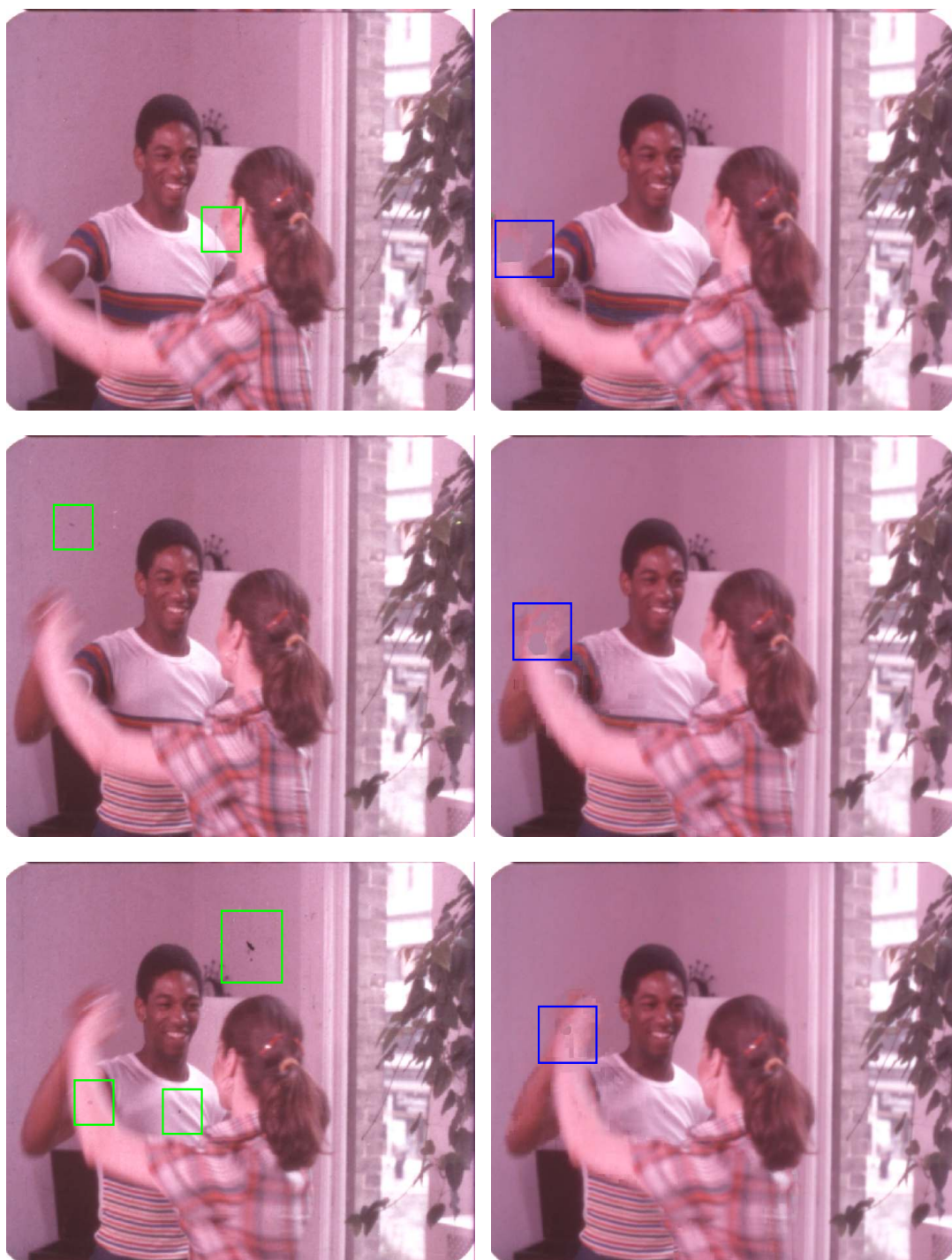
Figure 3.6: Processing three consecutive corrupted frames (left) with JONDI. Reconstructions are shown on the right. Blotches are shown in green on the left. As shown on the right all blotches are successfully removed. However, restoration artifacts are introduced in uncorrupted regions undergoing fast motion (shown in blue).
