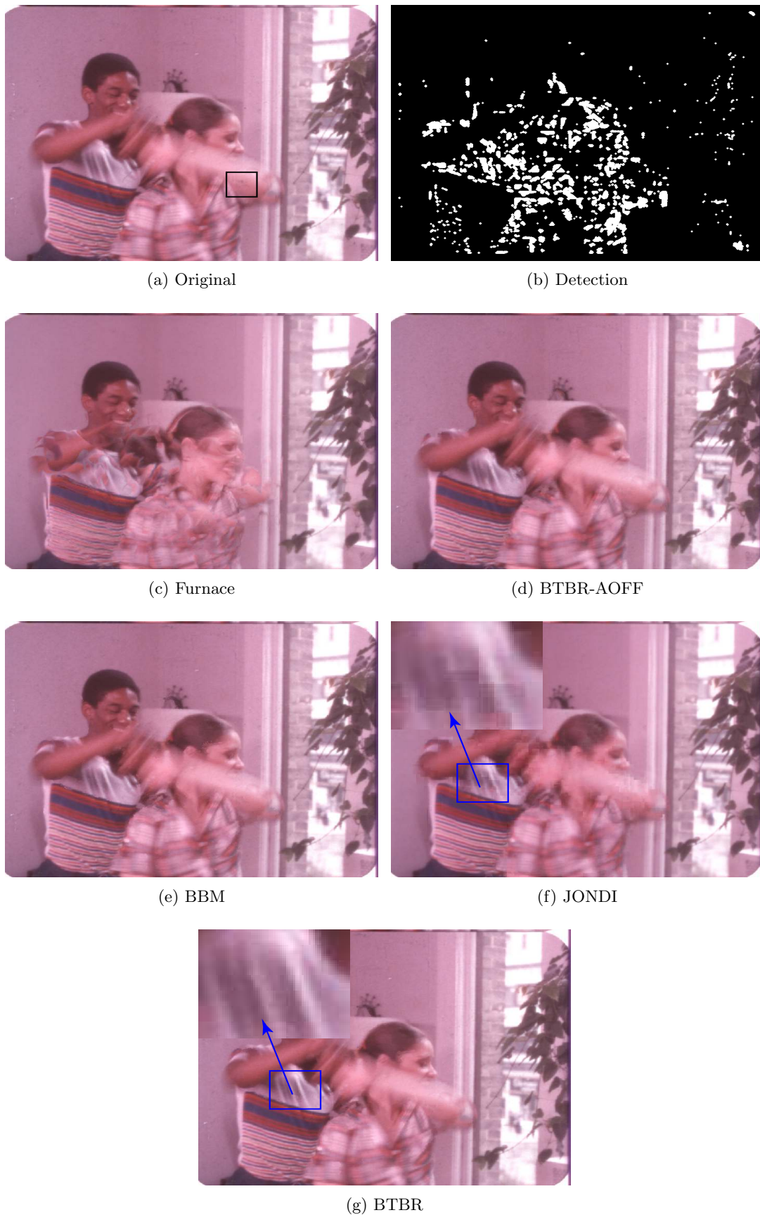
Figure 5.11: In clockwise direction: Frame 77 of DanceB1, its SDIp mask and reconstruction using different techniques. Blotches are shown in black boxes. JONDI generate reconstruction errors in regions misclassified as corrupted (shown in blue).
