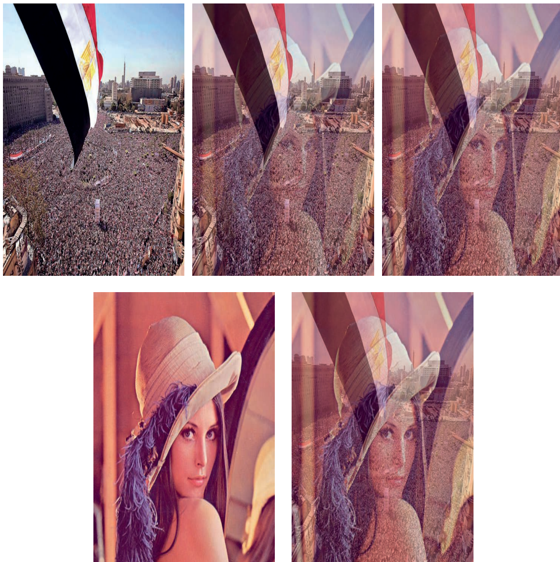
Figure 2.1: Mixing the image of lenna (bottom left) with an image of a crowd of people (top left) using equation 2.1 with different opacity values ( \alpha ). Here the crowd of people is the foreground while lenna is the background. Opacity values used (clockwise from top left) are \alpha = [1, 0.85, 0.5, 0.35, 0] . \alpha is fixed over an entire mixture. \alpha = 1 shows complete obliteration of the background (lenna) while \alpha = 0 shows complete absence of the foreground (the crowd)
