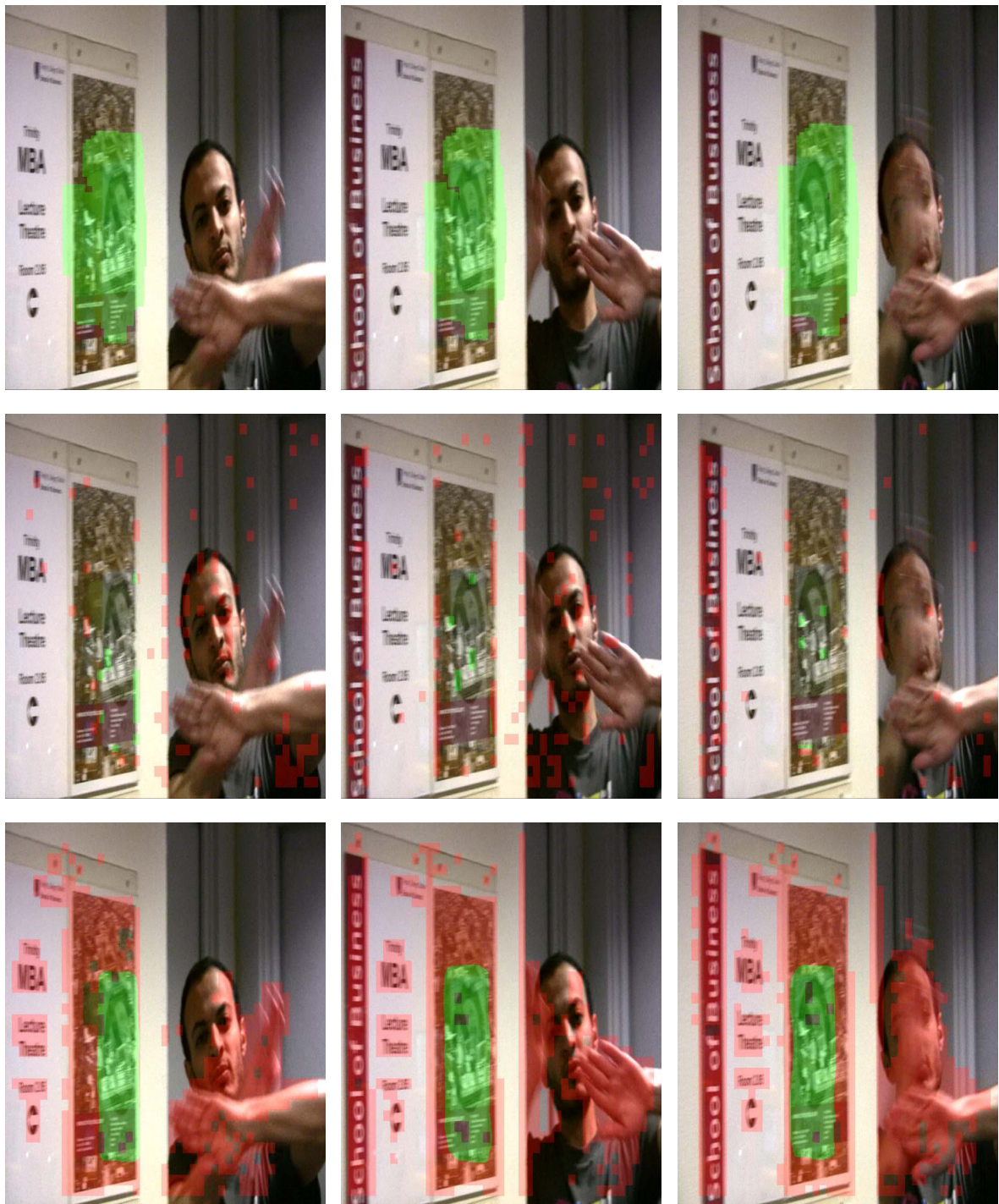
Figure 6.19: Reflection detection on SelimH using, from top; FEAPARD-F, SHARPNESS and DFD respectively. Correct detections are shown in green while false detections are shown in red. The pathological motion generated by the actor's hands is rejected by FEAPARD-F but detected by DFD.
