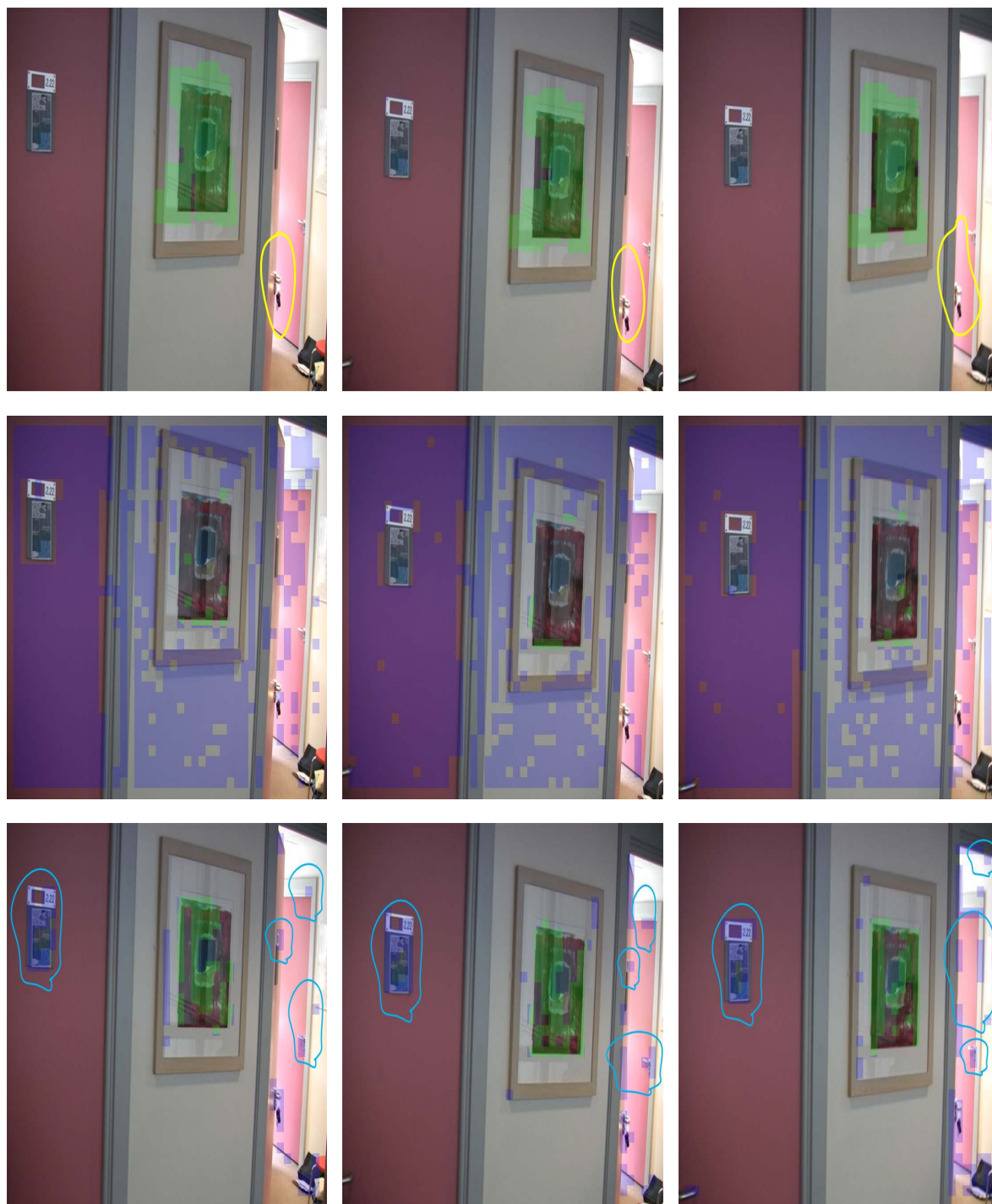
Figure 6.20: Reflection detection on PortraitA using, from top; FEAPARD-F, SHARPNESS and DFD respectively. Correct detections are shown in green while false detections are shown in blue. Some false detections are shown by blue circles (in the last row) for illustration clarity. SHARPNESS misclassifies flat areas as reflections and DFD misclassifies regions of occlusion (shown in yellow, first row) as reflections. FEAPARD-F however rejects flat areas and regions of occlusion.
