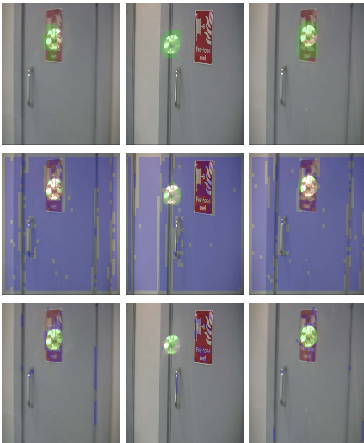
Figure 11.6: Reflection detection on Bulb using, from top; FEAPARD-F, SHARPNESS and DFD respectively. Correct detections are shown in green while false detections are shown in blue. SHARPNESS incorrectly flags flat areas as reflection.
