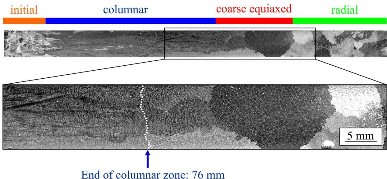
Fig. 2. Macrostructure of longitudinal section of CET sample prepared power-down technique at a constant cooling rate of 30 K/min.
