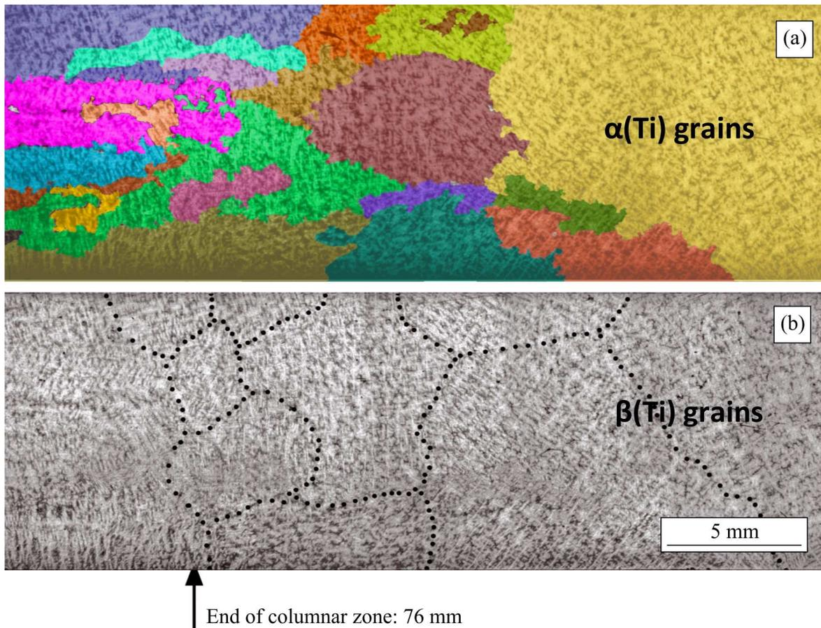
Fig. 3. Grain structure of a CET sample prepared by power-down technique at a cooling rate of 30 K/min: (a) columnar and equiaxed  $\alpha(\text{Ti})$  grains in the vicinity of CET, (b) columnar and equiaxed  $\beta(\text{Ti})$  grains in the vicinity of the CET.
