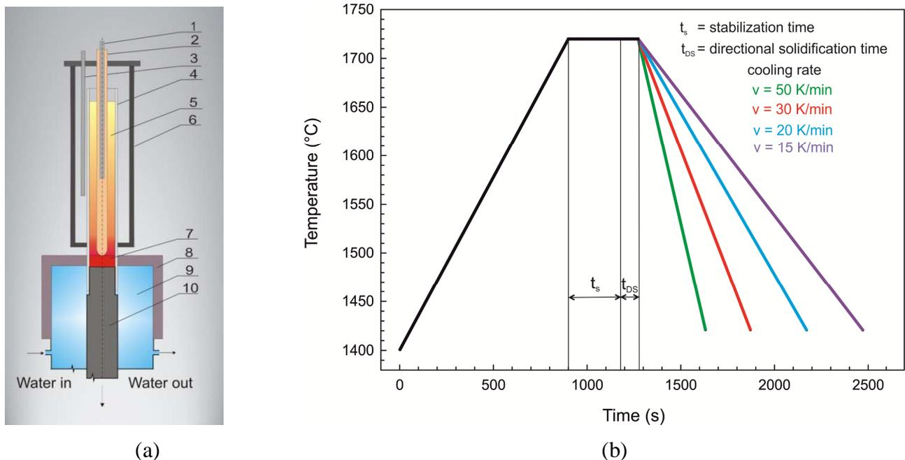
Fig. 1. (a) Schematic of the Bridgman type apparatus: 1 - measuring thermocouple, 2 - ceramic tube, 3 - control thermocouple, 4 -  $Y_2O_3$  crucible, 5 - solidifying sample, 6 - resistance heater, 7 - solid part of the sample, 8 - crystallizer, 9 - water bath, 10 - withdrawal rod. (b) Power-down experiments at four different cooling rates.
