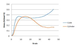
Fig 7. Typical stress vs strain behaviour of hemp concrete varying with specimen geometry.
