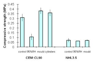
Figure 6. Effect of testing variables on compressive strength of concretes at 10 weeks. Control samples (100mm cube); cubes cured at >95% RH; cubes retained in moulds; cylindrical concrete specimens.
