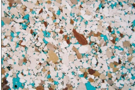
Figure 3. Manorhamilton sandstone with abundant quartz, little cement matrix and substantial pores. 2X polarized light
