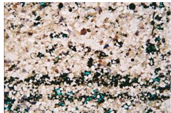
Figure 2. Drumbane sandstone: low porosity with clay mineral matrix and layered iron cement. X2 polarized light.
