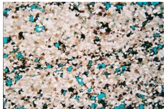
Figure 1. Drumbane sandstone: abundant clay matrix and significant iron cement and pores. X2 polarized light
