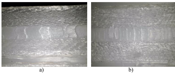
Figure 9: Machined surface for 20^\circ rake angle, highly worn tool, low depth of cut, a) low cutting speed, b) high cutting speed. Cuts performed from right to left
