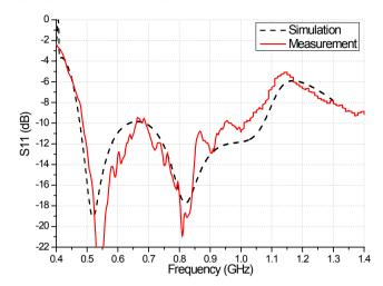
Figure 3. Simulated and measured S11 of the antenna.
