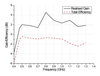
Figure 7. Realised gain and total efficiency of the antenna.
