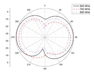
Figure 5. Elevation plane  $\theta$  = 0° plane radiation pattern at 500 MHz, 700 MHz and 900 MHz.
