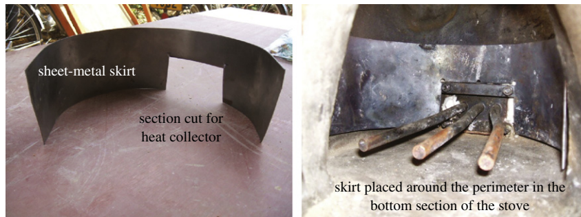
Fig. 9. Thin sheet-metal 'skirt' placed along the perimeter of the generator stove.
