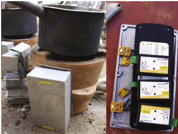
Fig. 13. Data loggers, enclosure and heat radiation shield.
