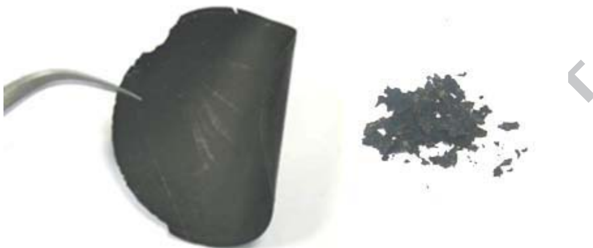
Fig. 1: Photo of free-standing PANi composite film (left) and PANi only film (right).
