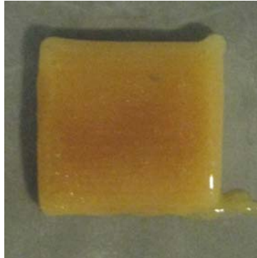
Figure 6: Resin with increased viscosity
