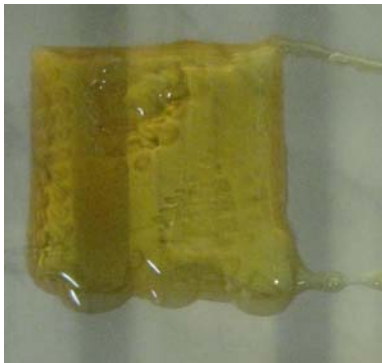
Figure 5: Deformation of low-viscosity resin
