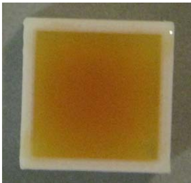
Figure 8: ABS support (white) containing cured resin
