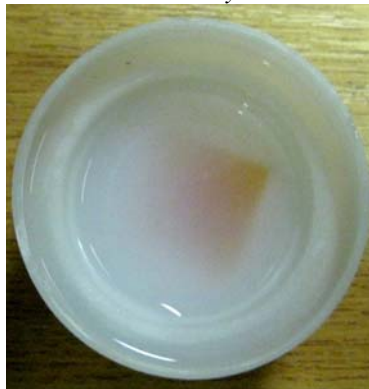
Figure 9: ABS dissolving in acetone
