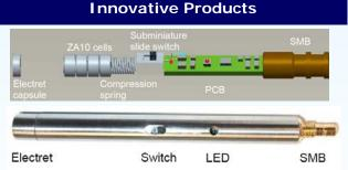
Figure 1: Low cost, high specification electret microphone
