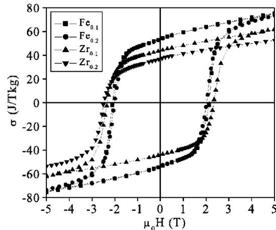
Fig. 1. Room temperature hysteresis loops of ball-milled SmCo<sub>6.6–x</sub>(Fe/Zr)<sub>x</sub>Ti<sub>0.4</sub>.
