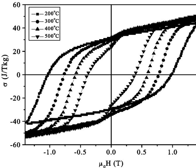
Fig. 2. Variation of coercivity with temperature in SmCo<sub>6.6</sub>Fe<sub>0.1</sub>Zr<sub>0.1</sub>Ti<sub>0.4</sub>.
