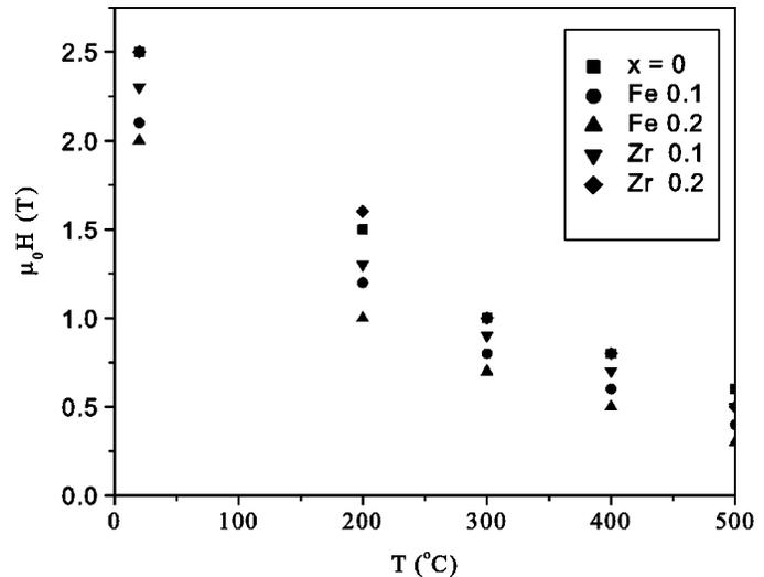
Fig. 3. Temperature dependence of coercivity in ball-milled SmCo<sub>6.6-x</sub>(Fe/Zr)<sub>x</sub>Ti<sub>0.4</sub>.
