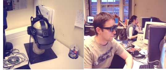
Figure 7(a). Standard dual LCD goggles (b). Polarized 3D Glasses
