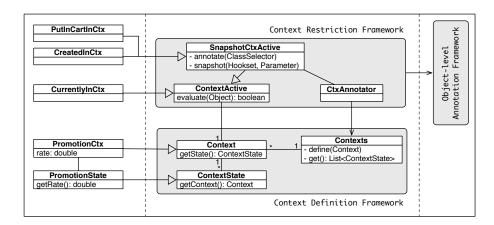
**Fig. 1.** The Reflex-based frameworks for context-aware aspects: the Context Definition Framework for defining when contexts are active and the Context Restriction Framework for defining context-dependent activation conditions.
