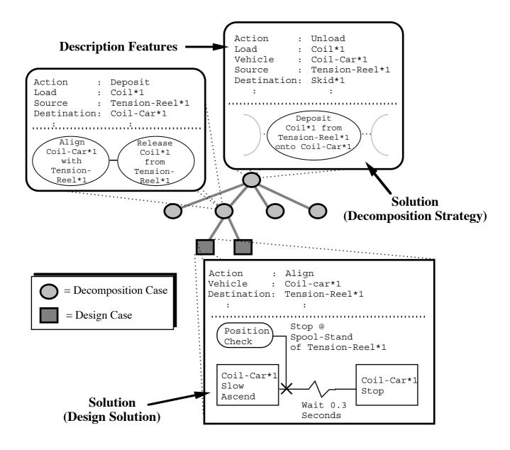
Figure 6. A plant-control design hierarchy.
