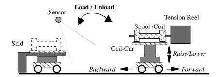
Fig. 1. Load/Unload Plant-Control Tasks
