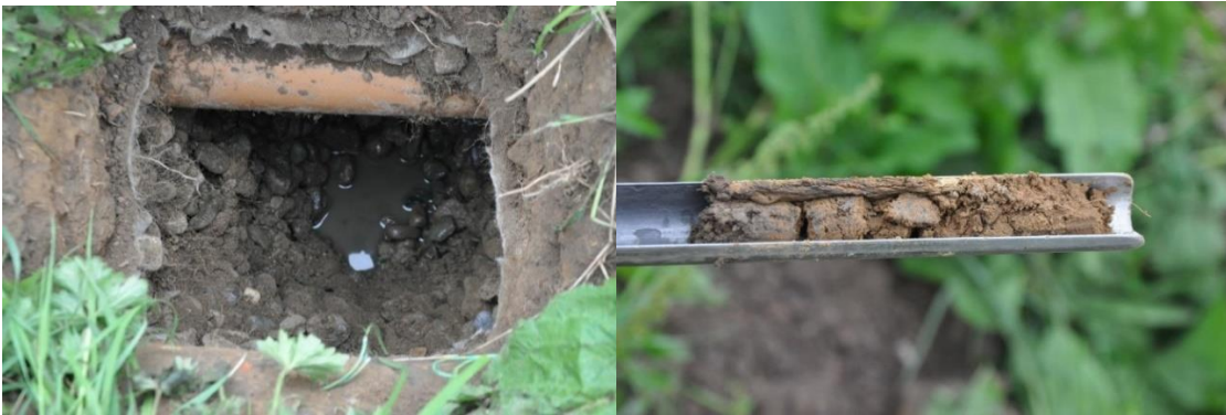
Figure SA2. (left) Accessing STU biomat, gravel matrix and percolation pipe visible (right) and using a corer.
