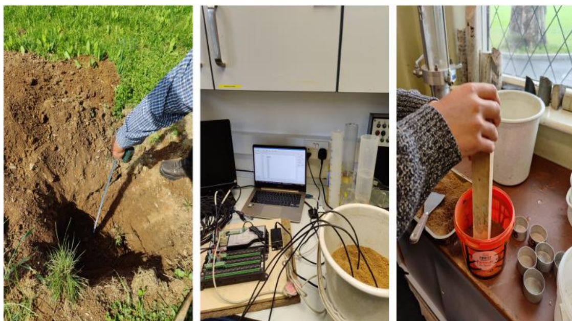
Figure 3.15. Subsoil retrieval for calibrations ensuring that sufficient depth is reached for a comparable soil matrix (left) calibration of EC5 sensors were used in triplicate (centre) and moisture was confirmed using wet dry weighing (right).
