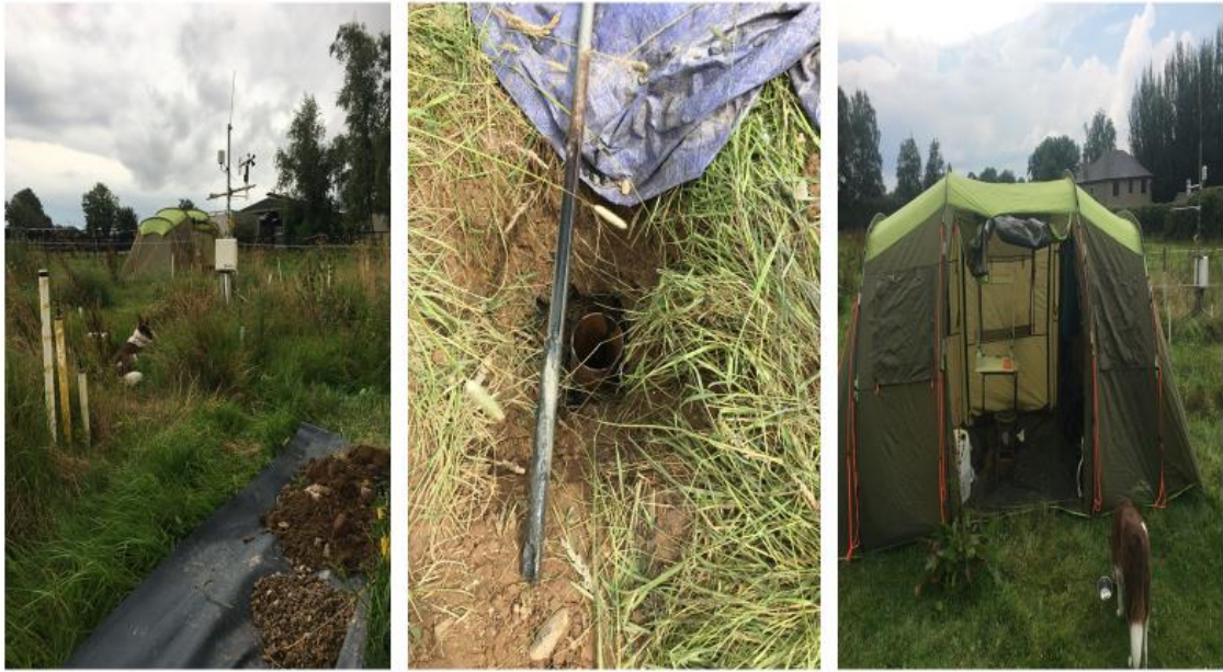
Figure 3.34. Subsoil excavation, with gravel and topsoil separation for effective refilling of cavities (left) subsoil core sample with dark black organic indicative of biomat growth (centre) temporary shelter for sample processing including a refrigerator for sample storage.
