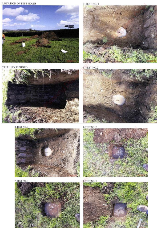
Figure SC1. The location of site suitability assessment in which percolation subsoil t-tests, and surface p tests are performed on site. T tests are performed 400 mm below ground level. Each whole is carved to set dimensions, filled and time measured for the falling head of water to percolate through the soil.
