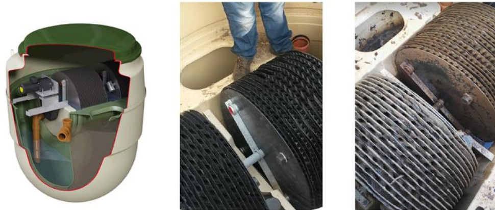
Figure 2.7. Klagester Biodisc RBC. Beginning left, shows the schematic of the RBC system including the integrated primary settling chamber, two-stage biozone, and secondary clarification chamber. The middle figure displays the device upon installation prior to the development of a biofilm. The figure right displays the device following 24 months of biofilm development, the bottom disks display stage 1 biozone and the upper biodisk displays stage 2, notice the colourisation differences between both biofilms.
