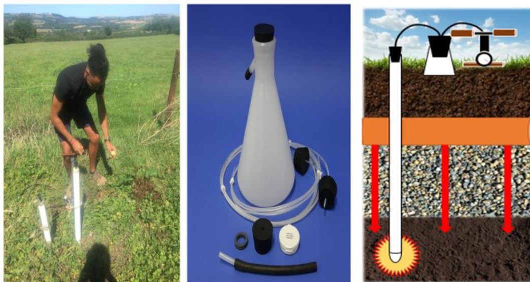
Figure 3.24. Priming lysimeters for sampling (left) porewater collection flask and collection tubing (centre) porewater collection diagram illustrating the flow of the effluent from the percolation pipe through the gravel, the direction marked with the red arrows towards the yellow area around the cup of the lysimeter shows the zone of influence is to be extracted using the Erlenmeyer flask and foot pump at the surface level (right).
