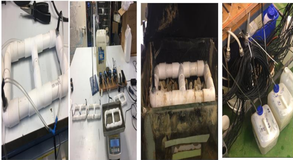
Figure 3.33. Soil column 8 shape manifold with peristaltic tubing (left) manifolds being calibrated with weighing scale and pump manifold (centre-left) manifold positioned within the column (centre right) influent reservoirs for PE and SE influent attached with peristaltic tubing (right).
