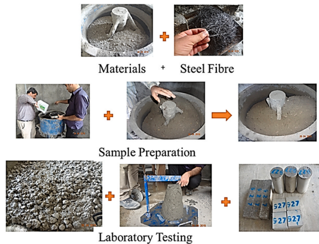
Fig. 5. Schematic plan of FRC mixture preparation.
