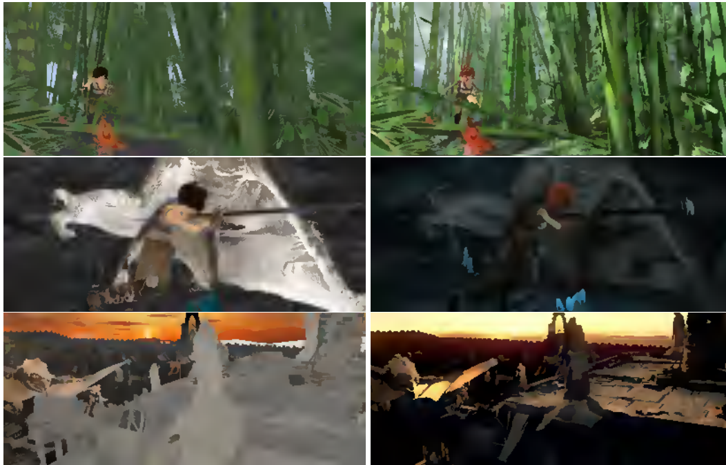
Fig. A.1 Sample frames from the SINTEL dataset. Albedo frames, which are flat, unshaded, surfaces exhibit constant albedo over time are seen on the left. Final frames which are full rendering with all effects including blur due to camera depth of field, motion and atmospheric effects (Butler et al., 2012)
