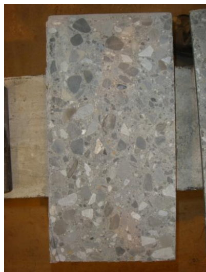
Figure 2.1 Smooth surface of C40/50 cylinder sample due to its dense microstructure
