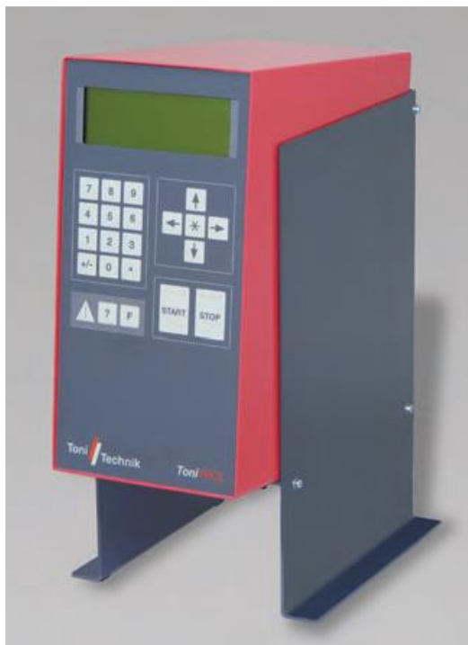
Figure 3.3 Control System of Young's modulus testing
