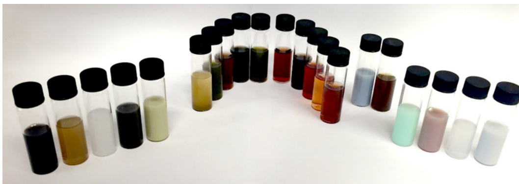
Figure 2.6: Some of the many materials that can be exfoliated using LPE, loosely grouped by type. From left to right: Group 1 is graphene, black phosphorous, hBN, TiB 2 , GaS; Group 2 is TMDs; Group 3 is transition metal oxides; Group 4 is transition metal hydroxides. Image unpublished at time of writing, used with permission.
