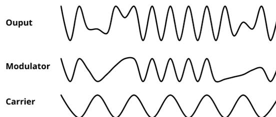
Figure 1: Example of the modulation of a carrier signal with a modulator.
