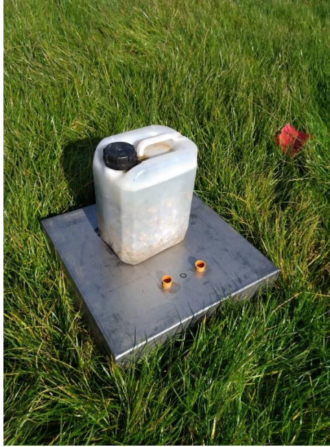
Figure 3. 3: An image of the static chamber design used in to measure N 2 O flux measurements in this study.
