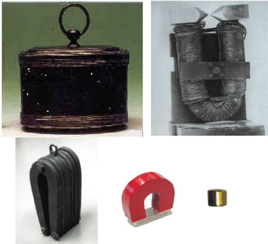
Fig. 6 Magnets from four centuries; top, seventeenth-century lodestone, nineteenth-century electromagnet; bottom, eighteenth-century horseshoe magnet, twentieth-century alnico and \text{Nd}_2\text{Fe}_{14}\text{B} magnets (not to scale)
