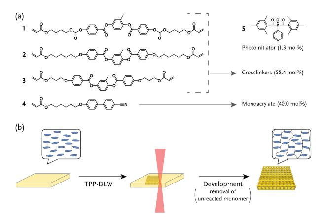
**Figure 1**. (a) Overview of reactive mesogens and photoinitiator used to prepare the LCphotoresist. (b) Schematic representation of the fabrication process for temperature responsive uniaxially aligned 3D microstructures. The blue rods represent the mesogens, which align along the longitudinal axis of the cell construct.
