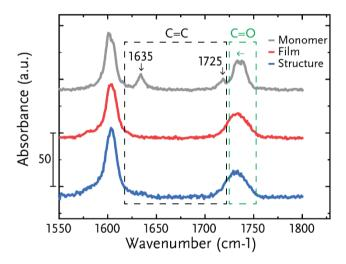
**Figure S4.** Confocal Raman spectroscopy of the LC-photoresist (or monomers), a fully polymerized film, and of a TPP-fabricated microstructure.
