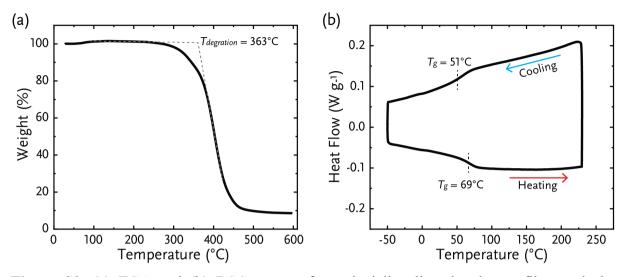
**Figure S2.** (a) TGA and (b) DSC traces of a uniaxially aligned polymer film made by photopolymerization of the LC-photoresist described in this work, exotherm up.
