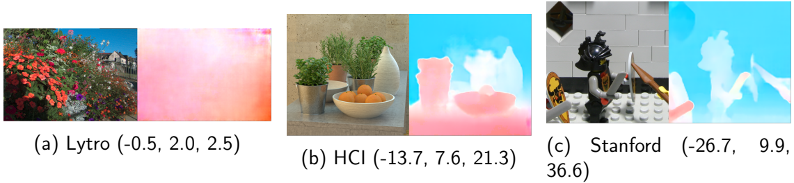
Figure 3.10: Disparity range ( d_{min} , d_{max} , d_{range} ) of Lytro, HCI and Stanford datasets ( \alpha = 4 ).
