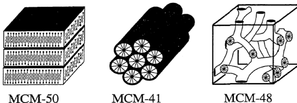
Figure 3.2: Schematic diagram of the M41S materials, MCM-50 (layered), MCM-41 (hexagonal) and MCM-48 (Cubic). Reproduced from ref 193 .
