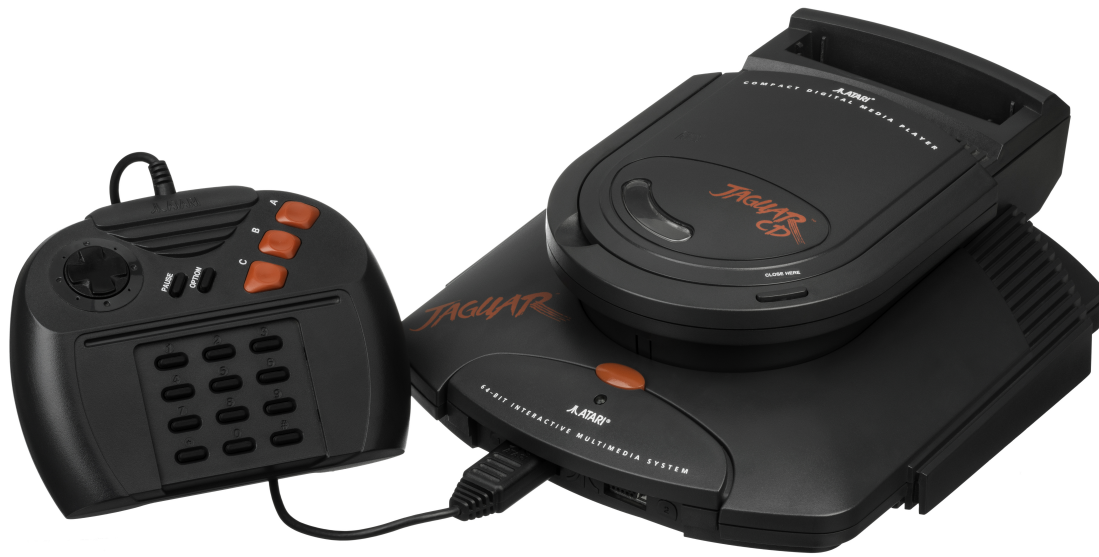
Figure 2: The Atari Jaguar with the Jaguar CD add-on in situ, along with the its idiosyncratic controller. The Atari Jaguar controller featured a telephone-style numeric keypad, which is used in the VLM to switch between visualizer presets. Source: https://commons.wikimedia.org/wiki/File:Atari-Jaguar-CD-wController.jpg . Accessed 14 July 2019. Credit: Released into the public domain by Evan-Amos.
