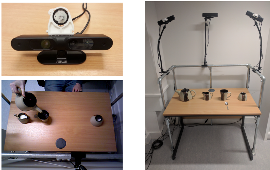
Figure 3.6: The arrangement of the recording set-up. Top-left image shows a vibration motor attached to an RGB-D camera (Asus Xtion). Right image shows the placement of the cameras in relation to the task table. Bottom-left image shows a colour image taken from the centre camera during a recording.
