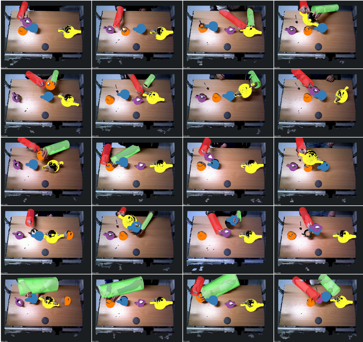
Figure 3.12: Pose estimation results for different sample recordings. In the first three rows, hand poses and object poses are estimated reliably. In the fourth row, object pose estimation errors are shown. These are due to misalignments of the cup due to changing topology and tracking losses due to complete occlusions. In the final row, arm pose estimation errors are shown. These errors are due to incorrect segmentation of left and right arm clusters when the hands are close together, and incorrect estimation based on inclusion of points from the subject's body.
