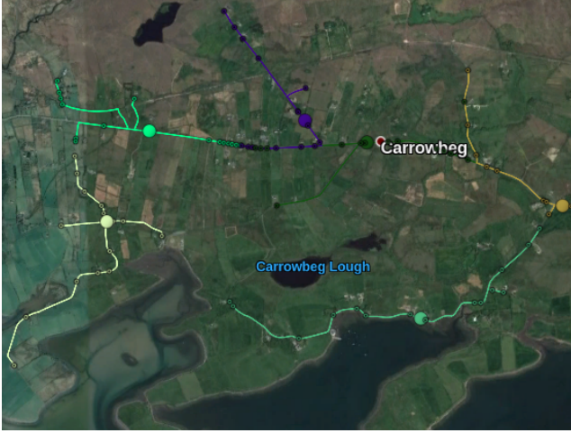
Fig. 5. Sample outcome of fixed-size single-stage clustering, a number of 16-size clusters assembling separate end-users groups. A 16-size cluster denotes a drop section equipped with 1x16 power optical splitter. Every round coloured sphere indicates a cluster centre and the place where drop cables can be branched off from a splitter.
