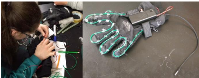
Fig. 4. Making the “EyeGlove” (left) with glued on Electro-Luminescence wire and audio cable to attach to phone for calls. Final prototype (right).
