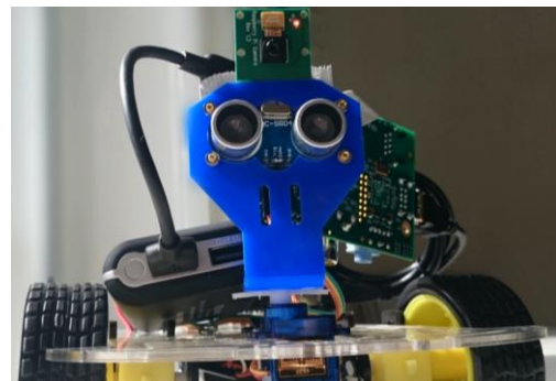
Fig. 3. "The Bridge Rover", the Raspberry Pi camera can be seen above the ultrasonic "eyes". A portable battery and Raspberry Pi computer can be seen connected in the background.
