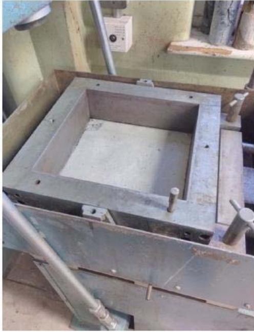
(a): Flat Interface Plate placed in the Shear Box
