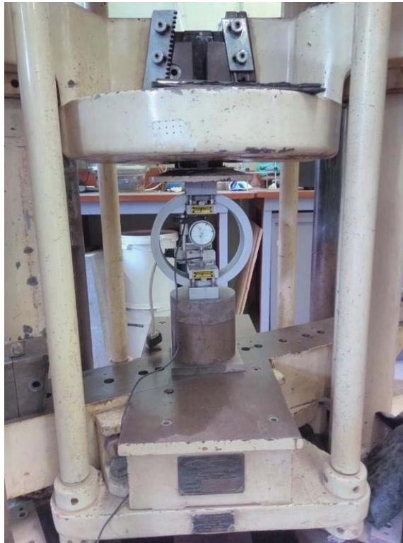
Figure 4-3: Calibration of proving ring using Denison Universal Testing Machine
