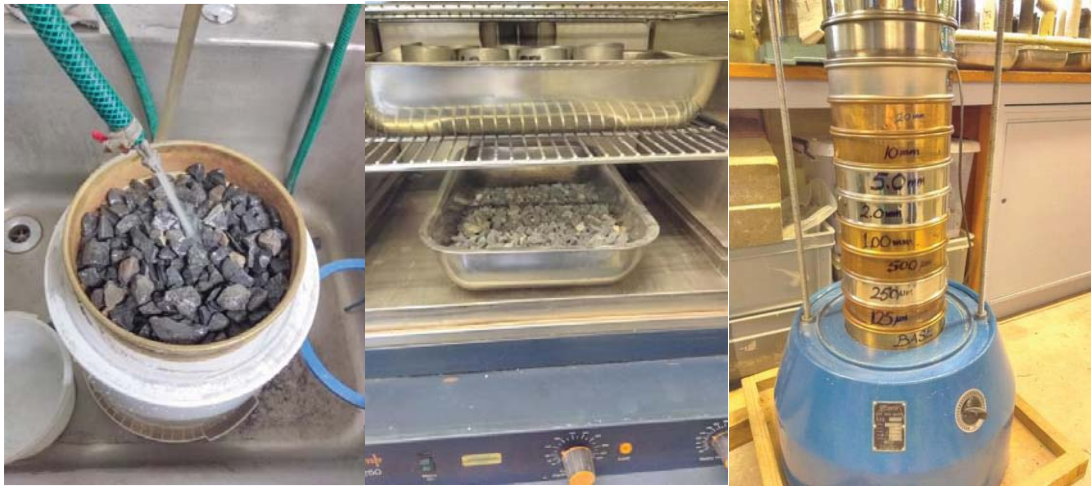
Figure 4-5: (a) Washing, (b) drying and (c) sieving of aggregates for preparing gradings 1-3
