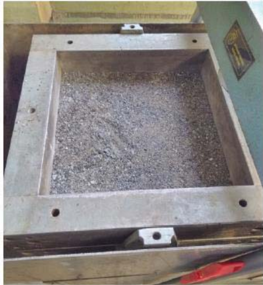
(b): Grading #1 Placed on top of the Serrated Interface
