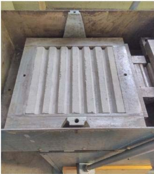
(a): Serrated Interface Plate in the Shear Box
