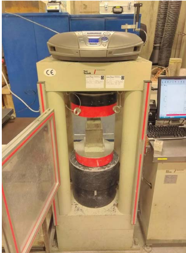
Figure 4-8: Concrete cube testing in Toni Technik Compression Machine
