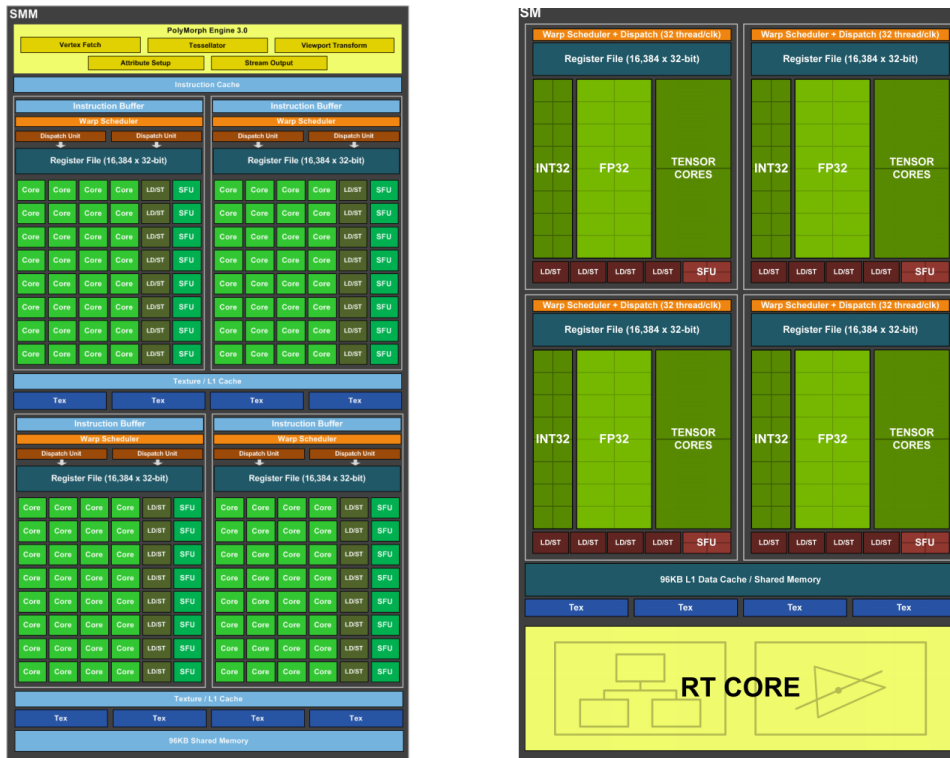
Figure 2.5: Comparison of the SMMs of Nvidia’s Maxwell architecture [39] (left) and Turing architecture [13] (right).
