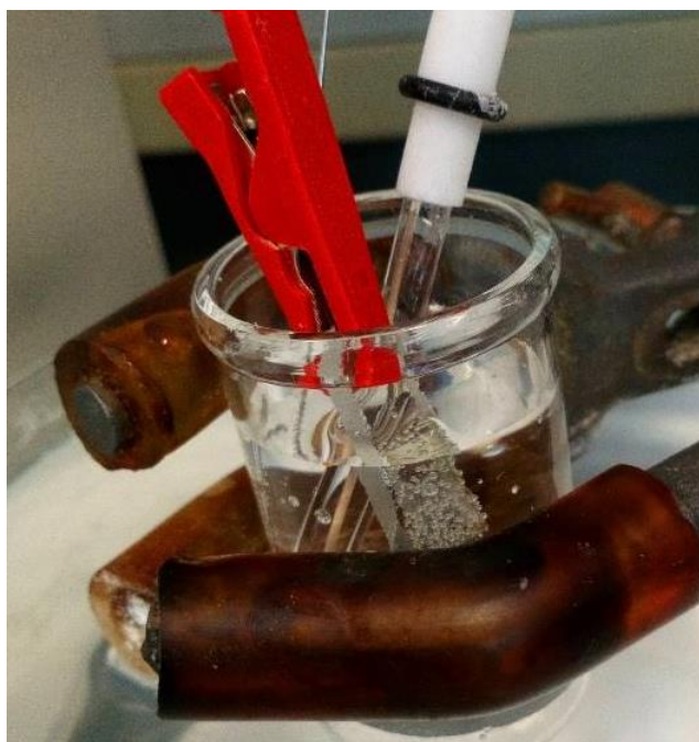
Figure 3.6.2: 2/FTO electrodes covered by O 2 bubbles during CV experiments.
