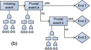
Figure 1. Generic representations of a fault tree (part a) and an event sequence diagram plus fault trees (part b).
