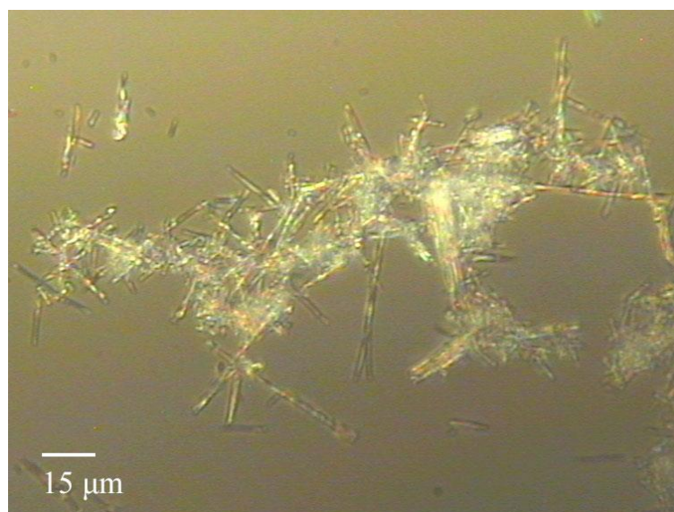
Figure 2.29: Phase contrast image of SiO 2 NWs embedded with BiFeO 3 and Fe 3 O 4 NPs.
