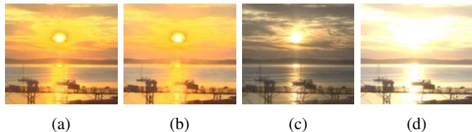
Fig. 15: Halo effect. (a) DeepTMO output, (b) DeepTMO trained with log-scaled values, (c) and (d) 2 top ranking TMO outputs.
