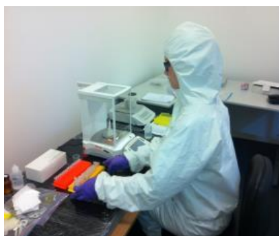
Figure III.27: weighting of the Travertine samples powder analysed by ICP-MS by Sylvain KM. and jean D., 2013
