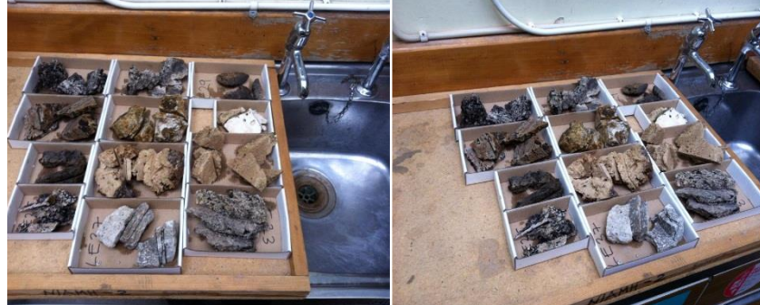
Figure III.20: Travertine Slices sample preparation, cutted, washed and dried by Sylvain K. M and Jean Dwyer in 2013
