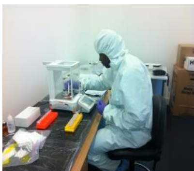
Figure III.27: weighting of the Travertine samples powder analysed by ICP-MS by Sylvain KM. and jean D., 2013
