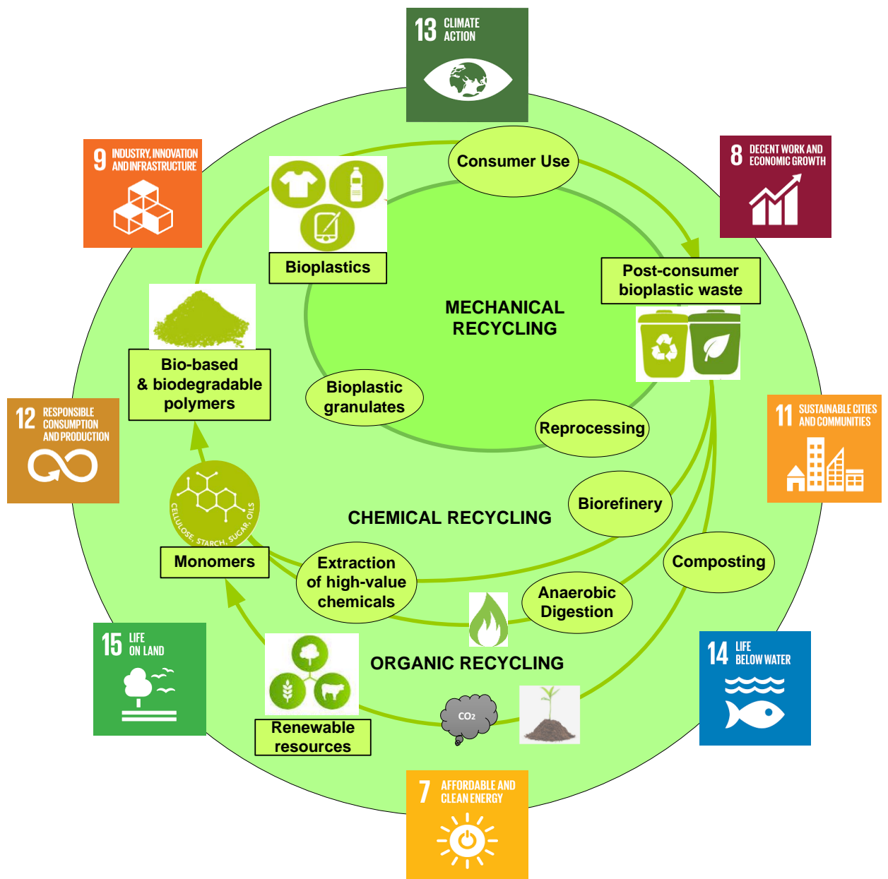
Figure 2. Schematic representation of recycling strategies for sustainable management of bioplastics and contribution towards SDGs
