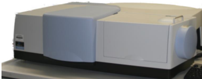
Figure 3.1. The Perkin Elmer Lambda 650, UV/Vis/NIR spectrophotometer with integrating sphere 150 mm, Trinity College Dublin.
