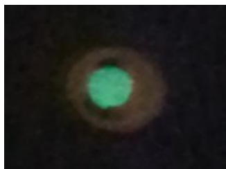
Figure 4.1. Final product phosphorescent phosphor ( \text{SrAl}_2\text{O}_4: \text{Eu}^{2+}; \text{Dy}^3 ) powder after being exposed to UV light (254nm) for 5 minutes.
