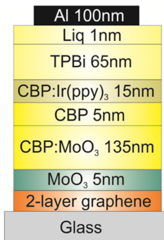
FIGURE 4.3: Schematic representation of the OLED structure. The graphene was transferred onto the glass and all subsequent layers were evaporated onto it. Everything but the graphene transfer was done by Philips corporation in Aachen, Germany.
