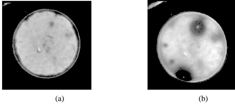
Fig. 3. Near-field image of sample B (a), before and (b), after degradation.
