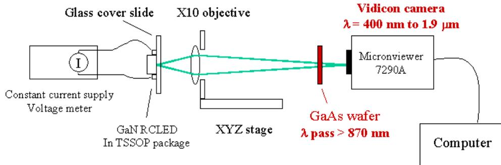
Fig. 4. Setup for imaging the thermal signatures of defect-related short circuits on circular contact RCLEDs. Because of the GaAs wafer, the green emission is blocked and the only wavelengths reaching the camera were infrared, between 870 nm and 1.9  $\mu\text{m}$ .
