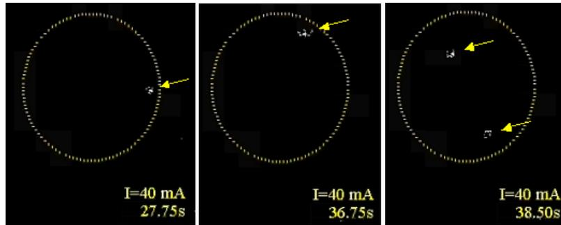
Fig. 5. Device A has transient hot spots that flash for less than 1 s. Dashed circles have been drawn in to represent the outline of the device [432 kB]. The movie shows that flashes start after ~24 s.
