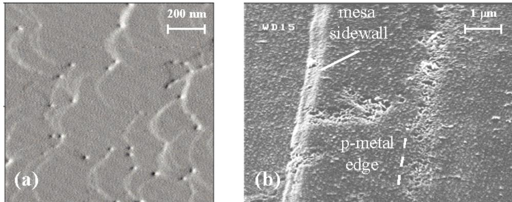
Fig. 6. (a) Typical  $1 \times 1 \mu\text{m}$  AFM image of GaN surface before degradation, showing open core dislocation density on the order of  $3 \times 10^9 \text{ cm}^{-2}$  and curved growth ledges. (b) SEM image after degradation and metal removal, showing large-scale surface pitting near the edge of the *p* metallization.
