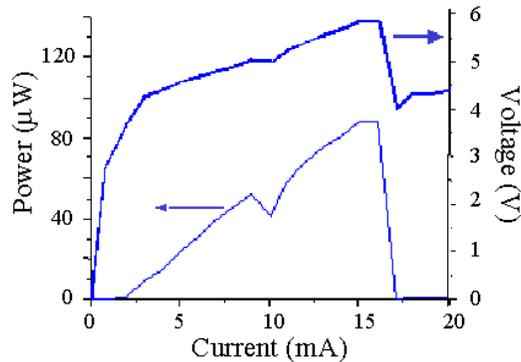
Fig. 2. LI curve for circular contact RCLED showing unstable light output.
