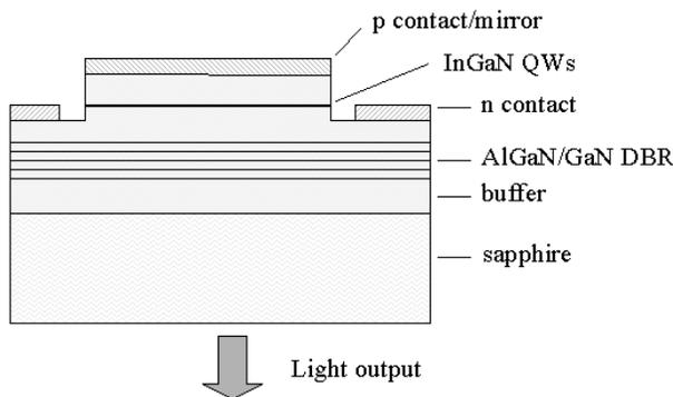
Fig. 1. Schematic of sample structure.
