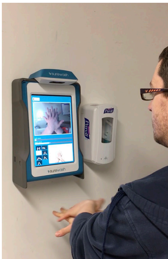
Figure 2. The SureWash GO simulator. The camera at the top of the unit measures the hand gestures and the feedback is provided via the screen. Note. The person in image 2 is Jonathan Ruttle, an employee of SureWash. Publication rights permission is appended to this file.
