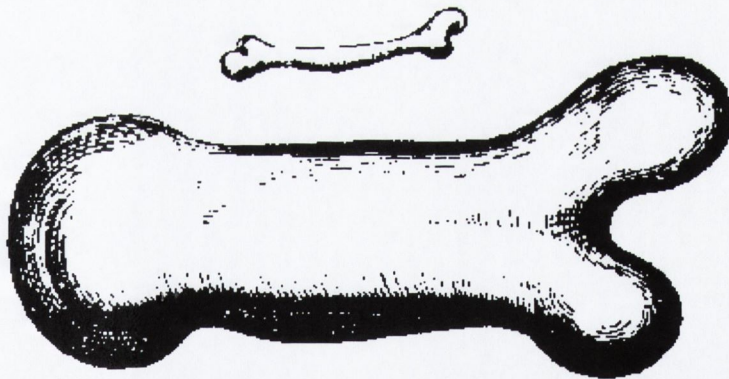
Fig. 5.1 A drawing by the Italian Galileo Galilei (1564-1642) demonstrating the dimensions of bones from animals of differing weights.
