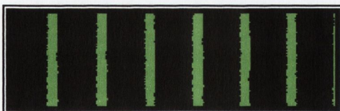
Fig. 5.17c: shows the green channel image after thresholded by the Colour recognition algorithm. Note the edge of the fringes is not perfectly straight, indicating some levels of noise.
