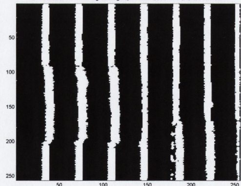
Fig.7.24b: The green channel image after all colour extraction in the Colour Encoded Recognition algorithm.
