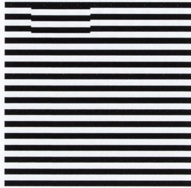
Fig. 4.48b: Synthetic image with 16 horizontal fringes
