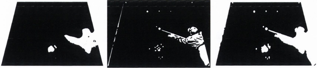
Figure 4.5: Binary maps. Left-to-right: (V(i, j) - R(i, j)) \leq 0 ; (V(i, j) - S(i, j)) \geq 0 ; ((V(i, j) - R(i, j)) \leq 0 \vee (V(i, j) - S(i, j)) \geq 0) .
